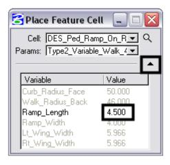
8. The cell is now ready for placement. The origin of the cell is at the curb face in the center of the ramp.
