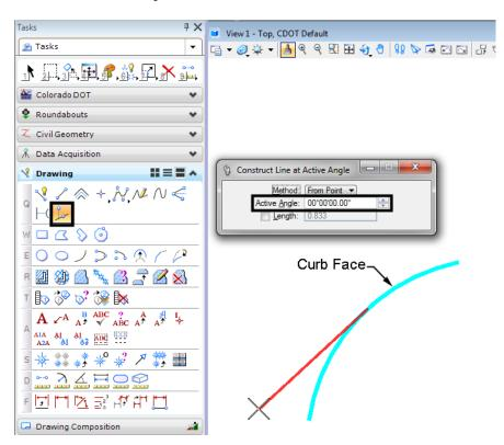
4. In the MicroStation Key-In window, type *active angle pt2* and press the Enter key. This is used to set the active angle to that of the line that was just drawn.
